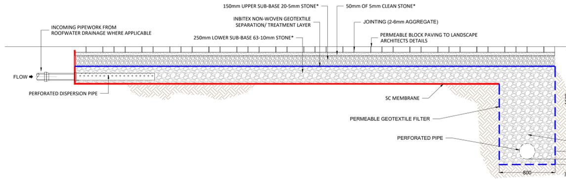
**TYPICAL PERVIOUS PAVING CROSS-SECTION**
